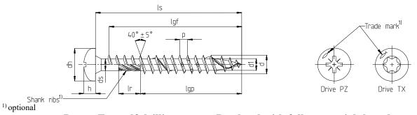
Power-Fast self-drilling screw - Pan head with full- or partial thread
