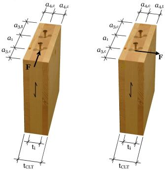
Table C1: Minimum spacing, end and edge distances of screws in the plane or edge surfaces of cross laminated timber
