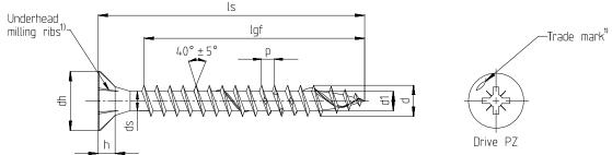
Power-Fast self-drilling screw - Small countersunk head with full thread
