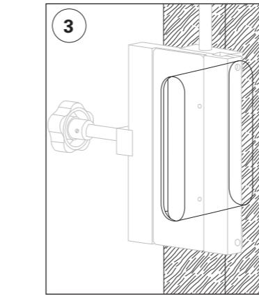
3. Mill the sash with a bit of 20mm.
